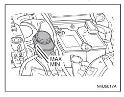
Turn the key off and then check the fluid level. The level should be between the MIN and MAX marks on the reservoir. If the level is below the MIN mark, add power steering fluid.
